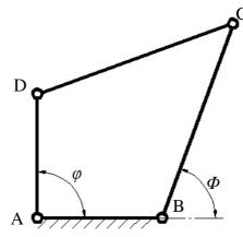
Fig. 1. Rhomboid mechanism with Galloway proportions of links
